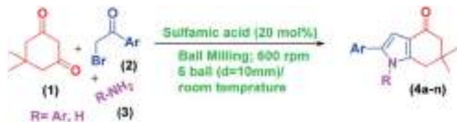
Scheme 2 General reaction scheme of sulfamic acid catalyzed for synthesis of 4-oxo-tetrahydroindoles scaffolds under ball milling conditions.
